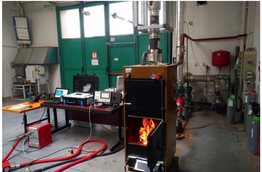
Figure 6: Laboratory examination of combustion equipment
