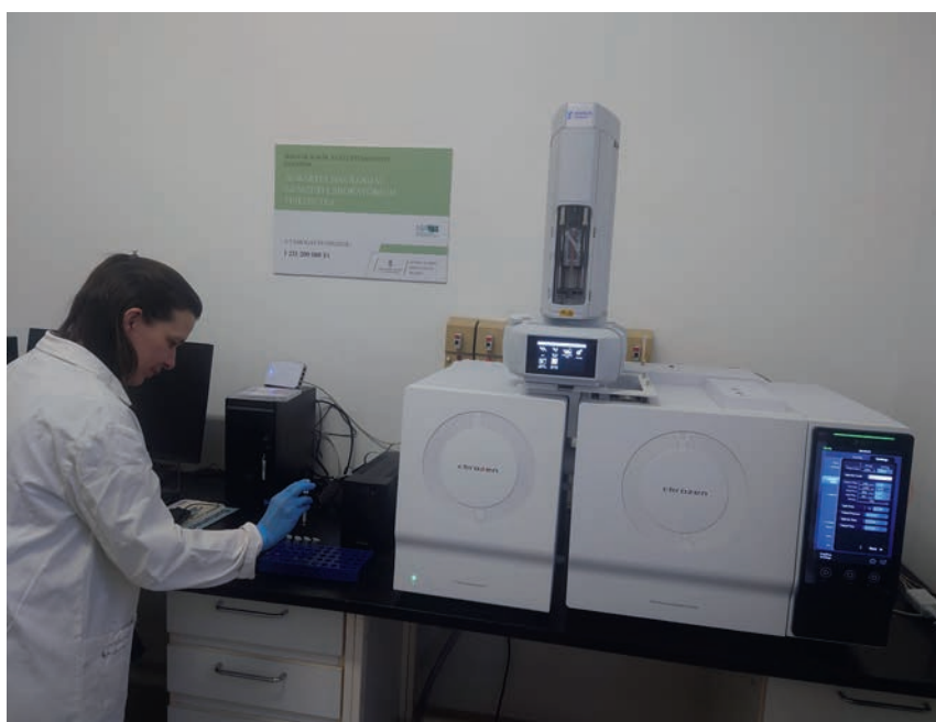
Figure 4: The newly acquired GC-MS instrument in the environmental analysis laboratory for the detection of organic micropollutants
